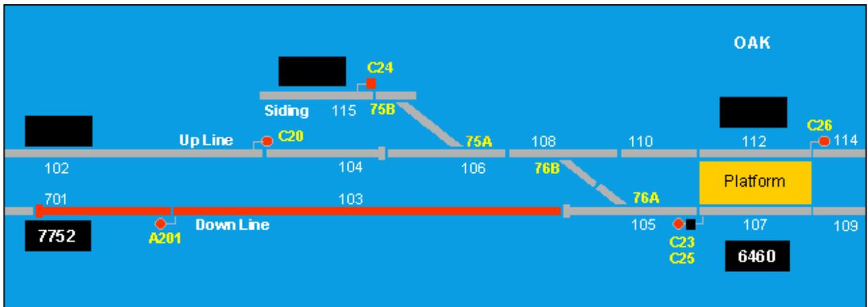
**Fig 5 - The train has released the points**
